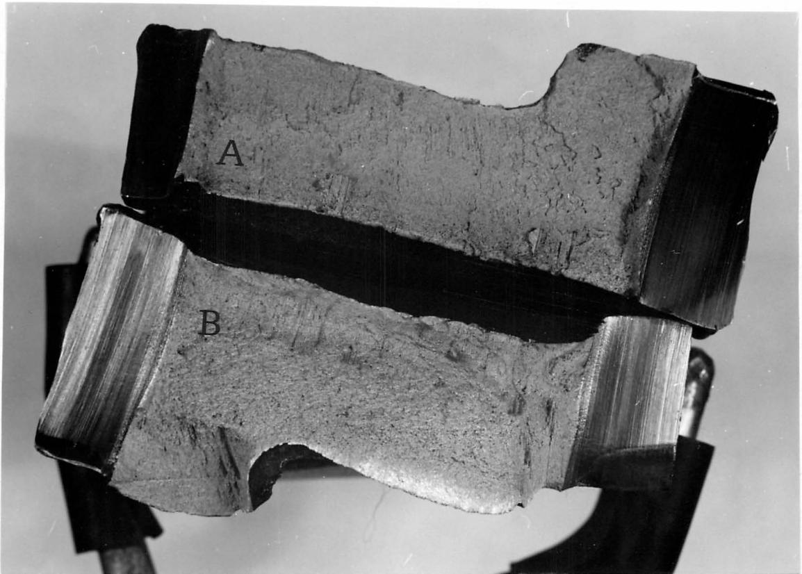
Figure 18. Fracture faces of two different flash welded joints made in Inconel 718.
