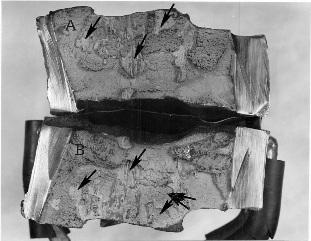
Figure 1. Macrograph of the mating fracture surfaces from a flash welded Hastelloy X sample. The arrows indicate the presence of flat spots. 1.5X
