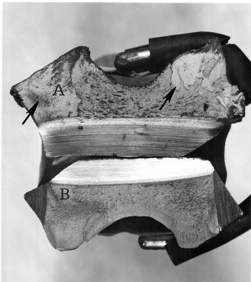
Figure 15. Fracture faces of two different flash welded joints made in Waspaloy.
